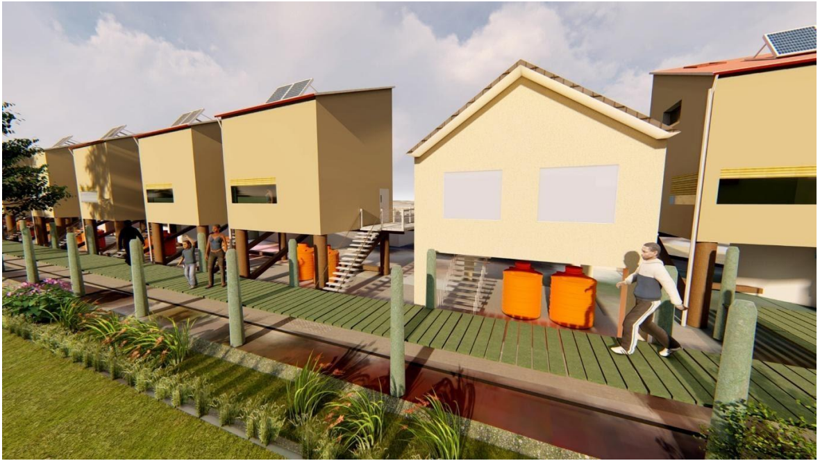
Figure 67. Elevated houses including a rain harvesting system, a boardwalk on stilts, and a bioswale
