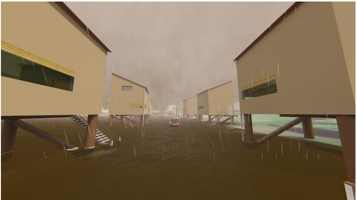
Figure 53. Elevated houses on stilts. This type of solution is preferable for future urbanization projects in areas with lower elevation, more exposed to floods
