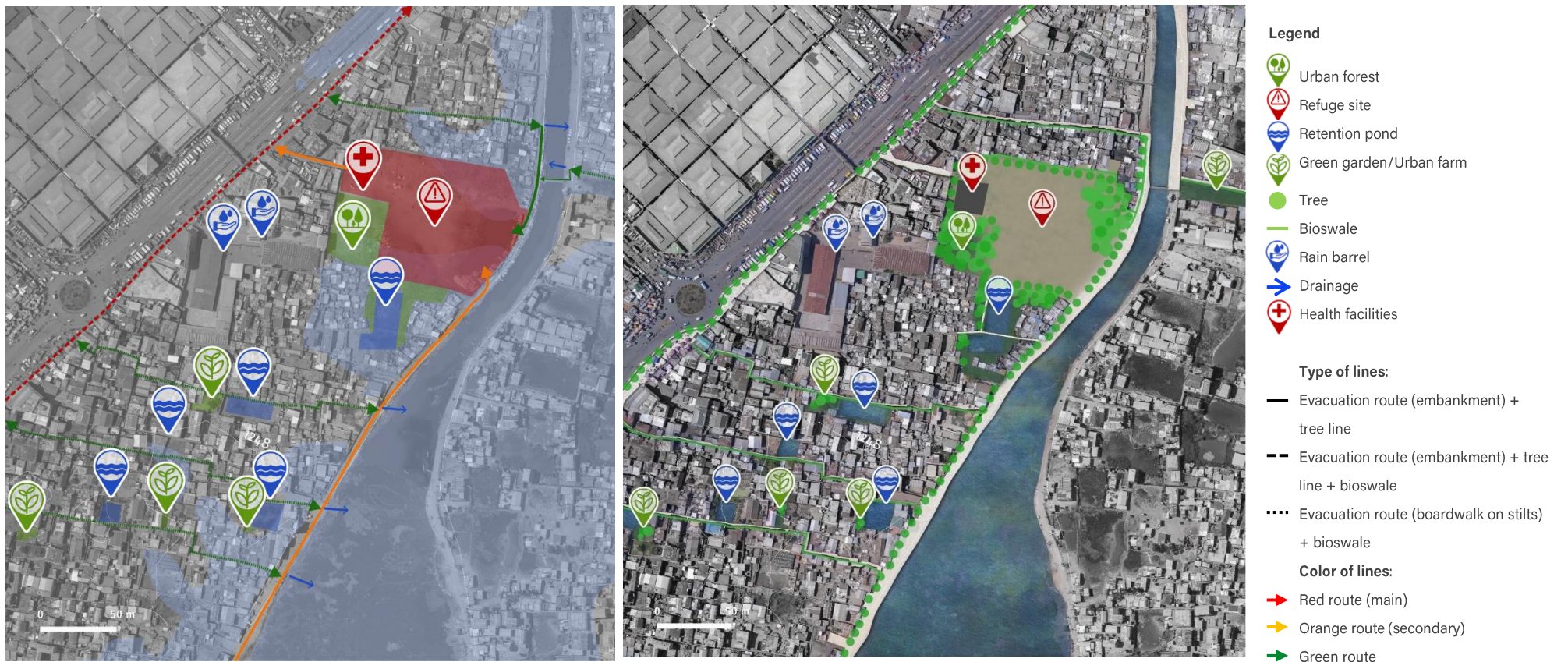
Figure 11. (left) Proposed NbS and complementary measures for flood risk reduction for site 3, including evacuation routes. (right) Plan for site 3
