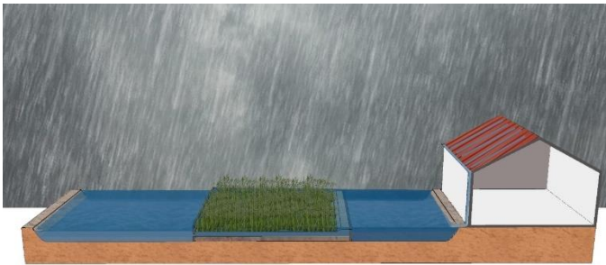
Figure 72. Inspiration image (section) of a helophyte retention pond
